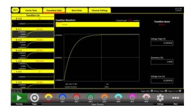
The software architecture provides the possibility to easily generate the patterns in different generation modality and also gives the opportunity to modulate the patterns with internal or external signals with the purpose to generate also different effects of noise (jitter, ripple, ...).
