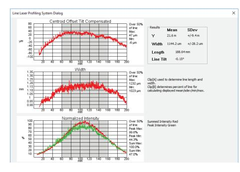
The line laser profiling system is supported by DataRay's full-featured, highly customizable, user-centric software which has no license fees, unlimited installations, and free software updates. The software controls the movement of the stage, automatically configures the optimal exposure time for the line laser scan, and provides an analysis of the line.
