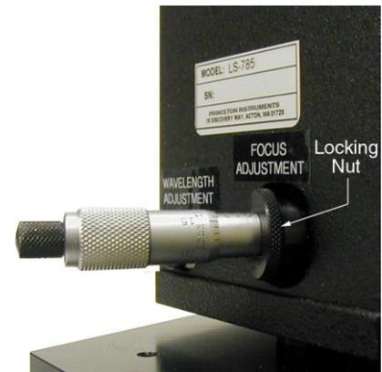
Figure 2-3. Focus Adjustment Micrometer
