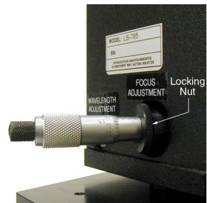
Figure 2-7. Focus Adjustment Micrometer
