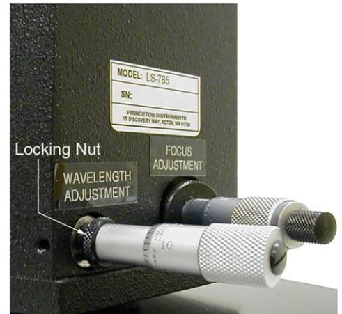
Figure 2-8. Wavelength Adjustment Micrometer
