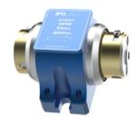
IPOptica's MPBB line of Faraday devices have been designed to minimum pulse broadening by unique short optical path length and low reflective indices. This results the great broadband wavelength protection to the ultrashort laser pulses at from 720nm to 950nm.
