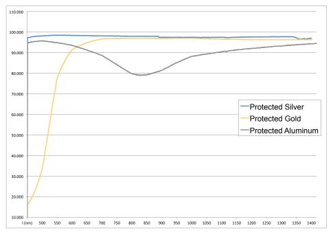
Typical Reflectivity vs. Wavelength Results for AOS Metallic coatings for OAPs
