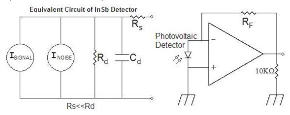
When background radiation shifts the operation curve by generating a constant output in the active element, the detector should be reversed-biased to bring it back to the optimum operating point: zero voltage.
