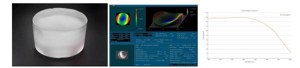
HEM® sapphire is the #1 leading sapphire material for highly sophisticated optical applications that require reliability, strength and a wide range of light transmittance. HEM Sapphire transmits light over a broad wavelength range spanning from 150nm to 5.5 microns.
