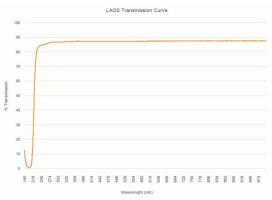
Crystal Systems has developed a special class of sapphire crystals called HEM® LAOS®, used for precision sapphire windows, sapphire lenses and sapphire filters. This material has shown the lowest absorption of all commercial sapphire materials available on a worldwide basis.
