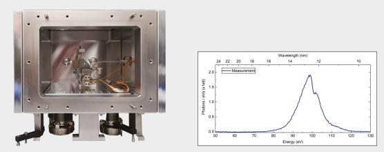
Up to 0.1 µW @ 3 kHz high-harmonic power in neon.
