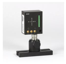
These detectors with integrated signal processing determine laser fluctuations with highest spatial and temporal resolution. The measuring principle allows for the inspection of single laser pulses. Thus, the position detectors enable the characterization and quality assurance of lasers. The detectors are equipped with LED displays for power level and x and y position.
