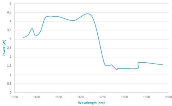
Zenith HP – Typical Signal Curve
