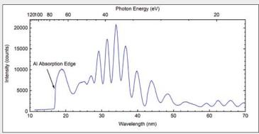
Top: Screenshot of our user-friendly software displaying the measurement of high-harmonic generated radiation in the XUV photon range.
